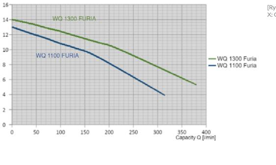
[Rys. Y: Head max H [m], X: Capacity Q [l/min]]
