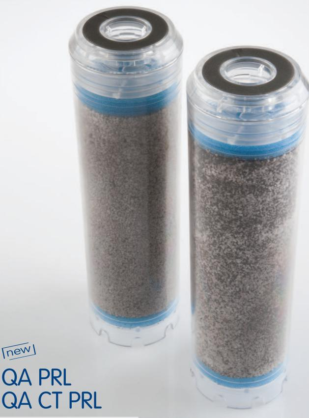
Range of filter cartridges with Pyrolusite for the reduction of iron and manganese. The combination with calcite allows also the neutralization of acid pH.
